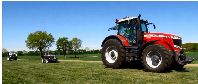
Fig. 2: Vehicles used to investigate formation control: a farm tractor Massey Fergusson 8680 leading RobuFast and Arocco mobile robots.
