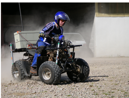
Fig. 1: Rollover prevention - test vehicles: quad bike Massey Fergusson MF400H (left) and grape harvester Gregoire G7-240 (right).
