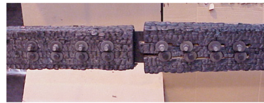
Fig. 1: Steel-to-timber joints in tension parallel to grain.
