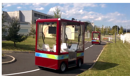
Fig. 2: (left) VipaLab vehicles used for the visual convoy. The first one is driven manually and the second one follows automatically in real time the leader's trajectory. (center) Comparison between the leader (blue) and the follower (red) trajectories (380m long). (right) Error between leader and follower trajectories (in cm). The 37 cm error (time 200) is due to the not flat road.
