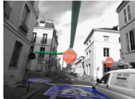
Fig. 1: Augmented reality from a constrained SLAM algorithm. A prior map is used to superimpose information related to the way to follow or traffic signs.
